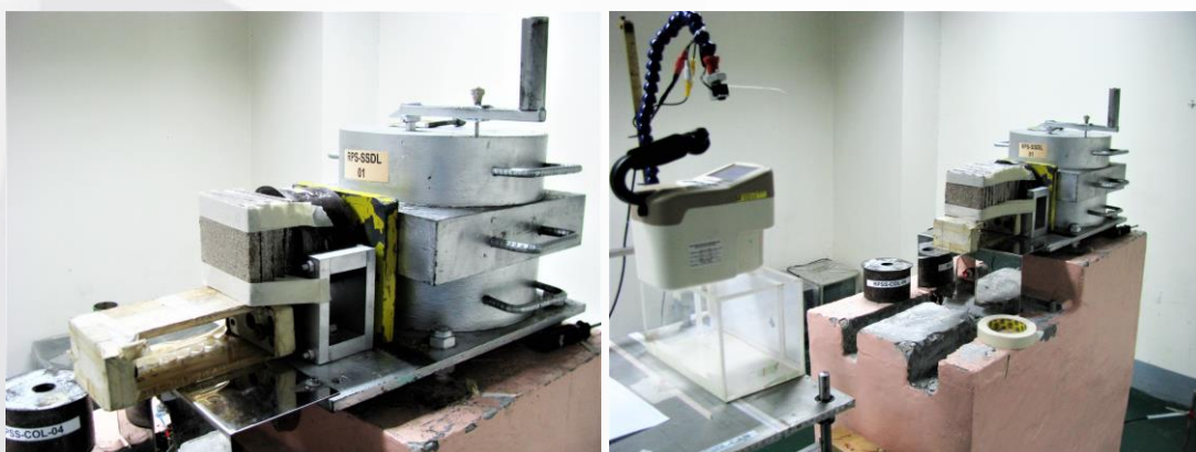
Samples placed in front of the Cs-137 irradiator for shielding effectivity testing. A doserate meter placed at a fixed distance from the source to measure the effectivity of the samples.
