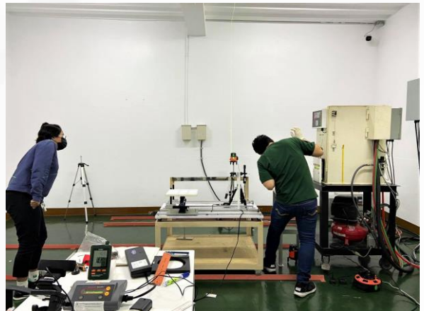
SSDL Staff positioning copper filters along the x-ray beam for field HVL measurements according to ISO 4037:1996 Narrow Spectrum Series.
