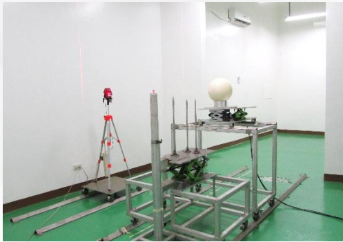
Reference He-3 spherical proportional counter in a 10" Bonner sphere measuring total field counts in a bare Cf-252 field.
