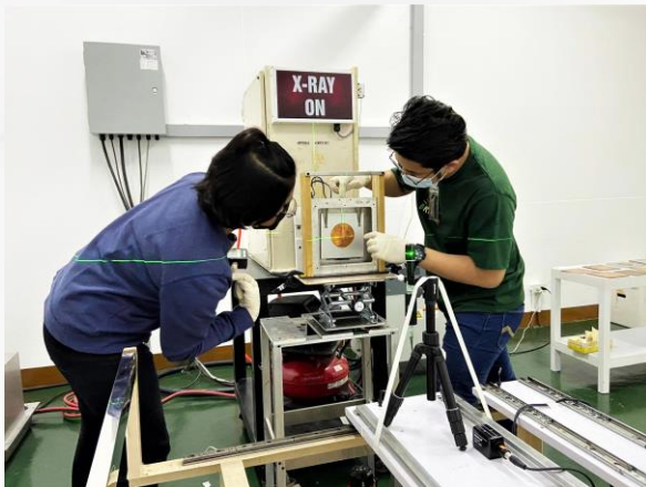
SSDL Staff positioning copper filters along the x-ray beam for field HVL measurements according to ISO 4037:1996 Narrow Spectrum Series.
