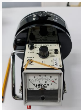
Reference beta survey meter traceable to a primary standard laboratory (AIST)
