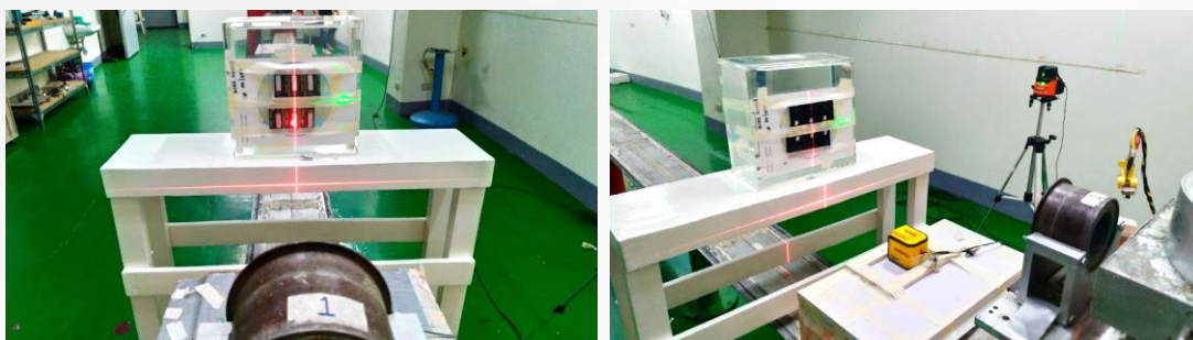
Personal dosimeters being irradiated for blind testing of personal dosimetry systems (Left: Optically-stimulated luminescent dosimeters; Right: Thermoluminescent dosimeters)
