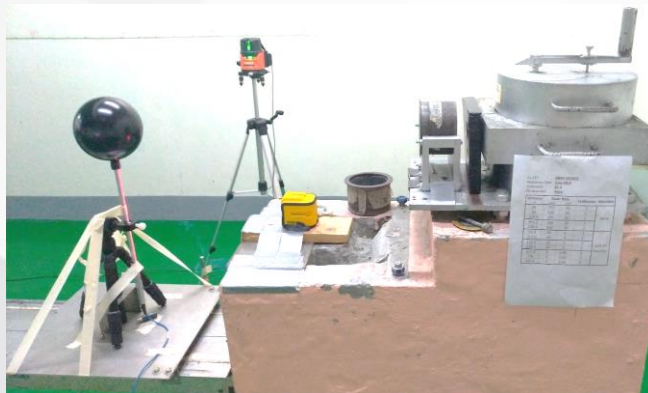
Reference 1-L spherical ionization chamber measuring kerma in the Cs-137 field.
