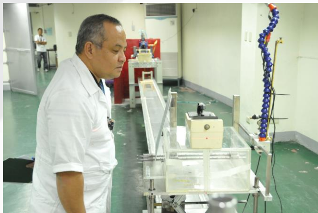
SSDL staff positioning a survey meter in the Cs-137 field for response determination.
