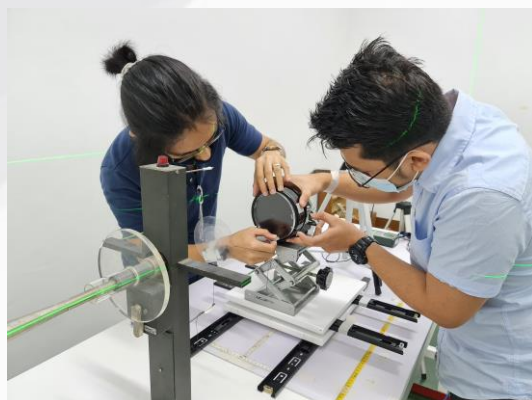
SSDL Staff removing the build up cap of the reference instrument for beta radiation field measurements.
