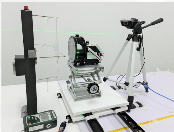
Standardizing the beta radiation field for ambient dose equivalent H^*(0.07)
