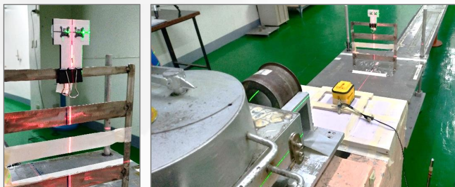
IAEA Postal Audit (2020) OSLDs irradiated in air at 1 meter from the Cesium-137 radioactive source for reference air kerma measurements.
