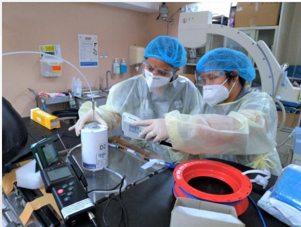
SSDL staff positioning the reference brachytherapy chamber for source output measurement
