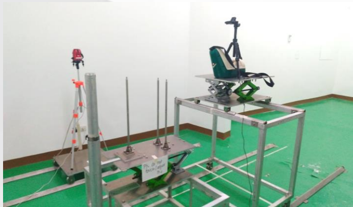
Neutron survey meter in the total field of the bare Cf-252 for response determination
