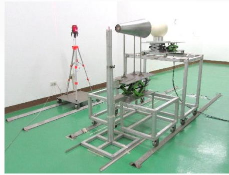
Reference instrument measuring scattered field counts using the shadow cone.
